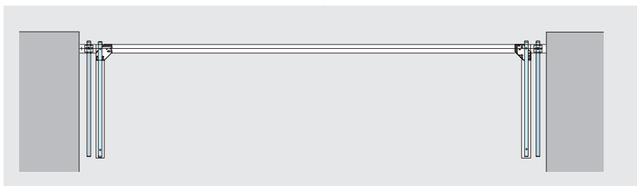
Stacking with one stacking leg for sliding panels in front of the pivoting end panel, single- or double-action, on each side (2 pivoting end panels/2 sliding panels).
